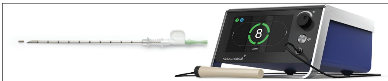
Figure 1: Left: Pintuition marker and Pintuition Needle. Right: Pintuition detector consisting of the Pintuition probe (front) and base unit delivering auditory and visual feedback to guide seed detection
